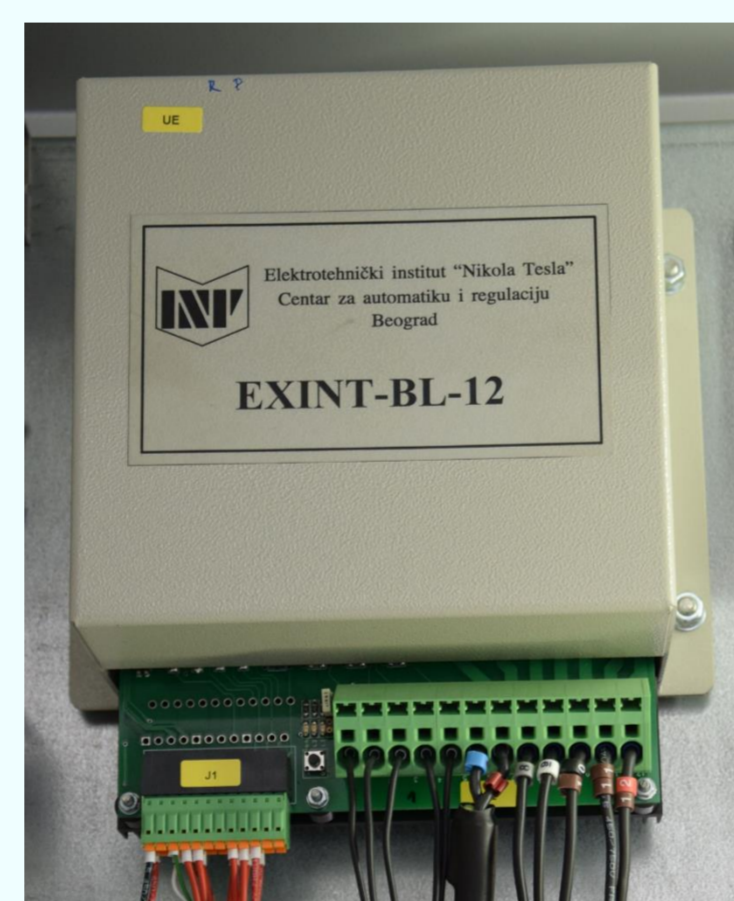
AVR for brushless excitation system, I_{fn} = 12A
