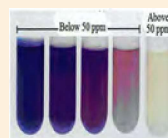
PCB test kit – Chlrine content in the oil LDX Analyzer
